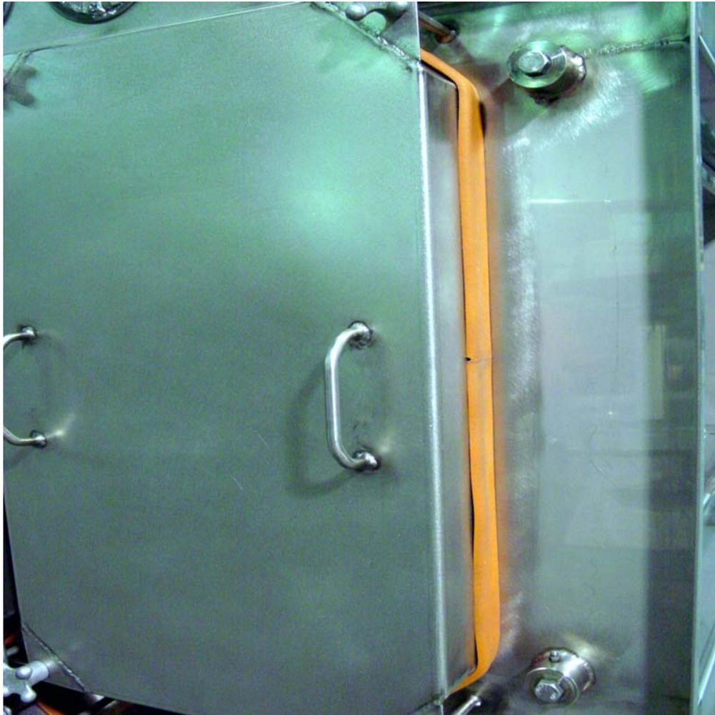
(top and bottom drive bolts located on right side of unit)
