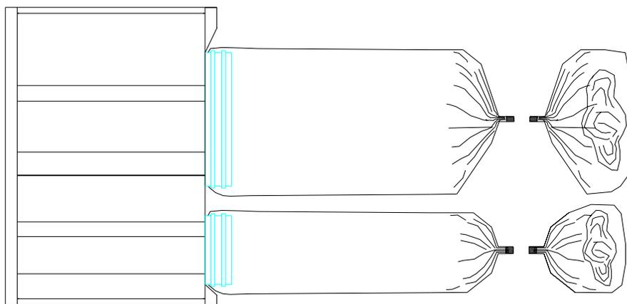
(residual filter bag stubs shown of both prefilter and HEPA filter)
